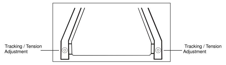
Note: Adjustment is through small hole in end
